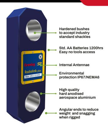
Crosby Straightpoint Radiolink Plus is designed to be rigged with Crosby standard shackles - DNV-GL type approved wireless tension load cell capable of weighing and dynamic load monitoring in capacities from 1t to 300t – from stock with an ATEX and IECEx version available for hazardous areas, zones 0, 1 & 2.
